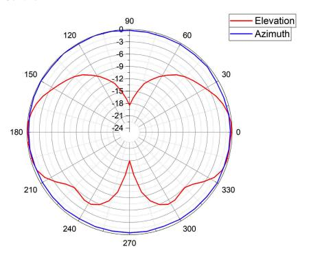
Frequency: 4.65 GHz Max Gain: 4dBi
